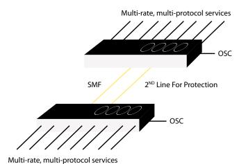
Services are converted to specific wavelengths and multiplexed together onto a single fiber, then demultiplexed at the destination.
